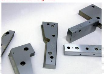
Surface grinding of the plant, base and active side
