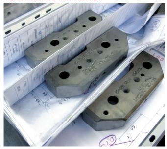
Complete fabrication - cutting edges, knife joints and wire eroded fitting holes
